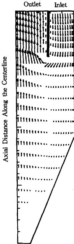
Fig. 7. Computed Velocity Vector for Axial Type Inlet.
