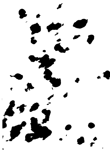
Fig. 5 Transmission electron microscope (TEM) photograph of soot deposit
