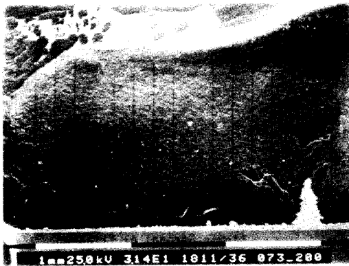
(a) fracture surface of the SiC/SiC joint with Ag-9at%Ti alloy
