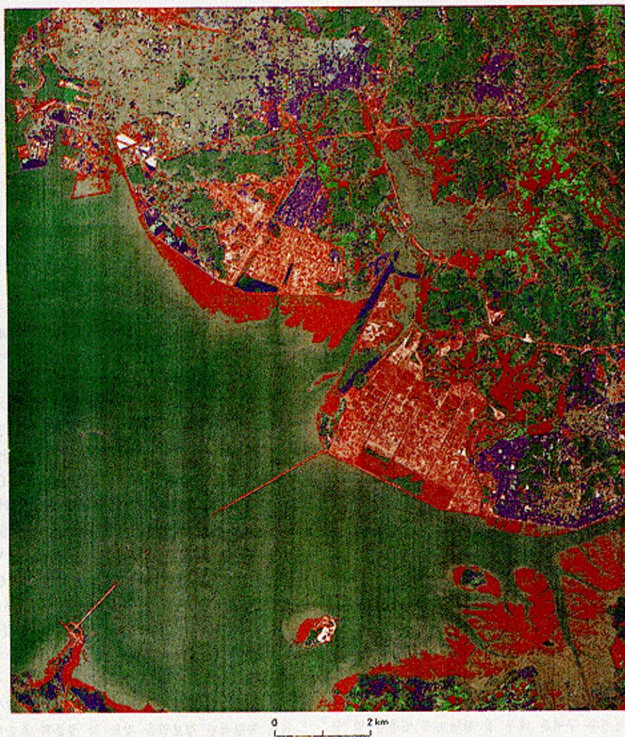
Fig. 10. Color composite image of the resulting change vector; the background image represents band 3 of LANDSAT TM data acquired on September 22, 1995.
