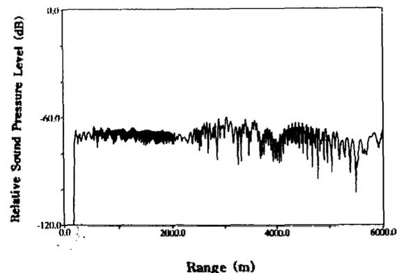
Fig.8 Relative sound pressure level versus distance at 200 Hz when the acoustic source and receiver are located at 1450 m and 500 m from the water surface, respectively.
