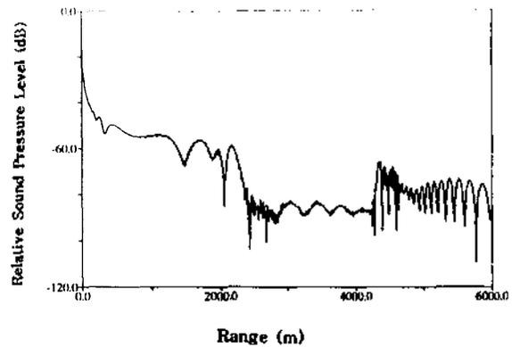
Fig.7 Relative sound pressure level versus distance at 200 Hz when the acoustic source and receiver are located at 1450 m from the water surface.
