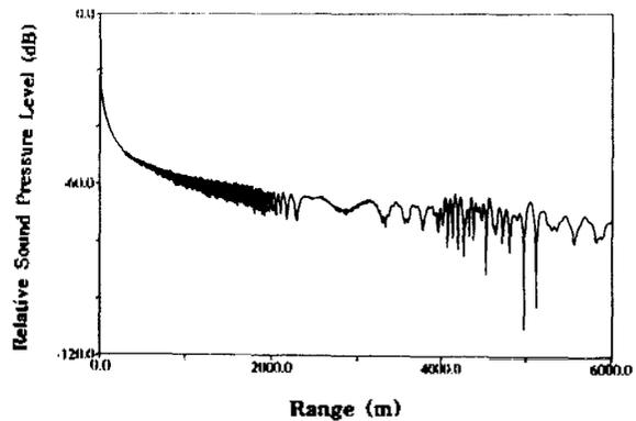
Fig.10 Relative sound pressure level versus distance at 200 Hz when both of the acoustic source and receiver are located at 500 m from the water surface.
