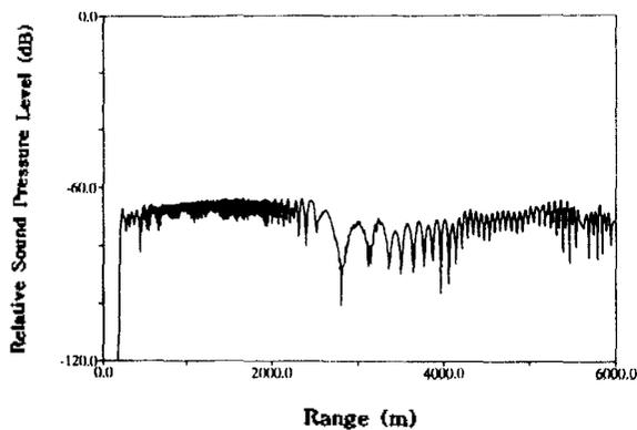
Fig.9 Relative sound pressure level versus distance at 200 Hz when the acoustic source and receiver are located at 500 m and 1450 m from the water surface, respectively.
