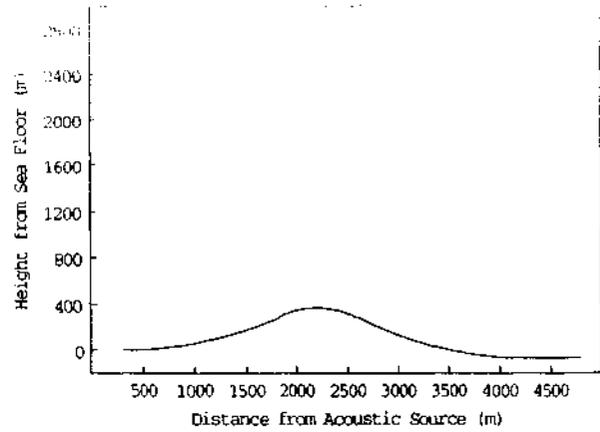
Fig.6 The geometry of sea mountain for calculation. The water surface is placed at 1500 m from the sea floor.
