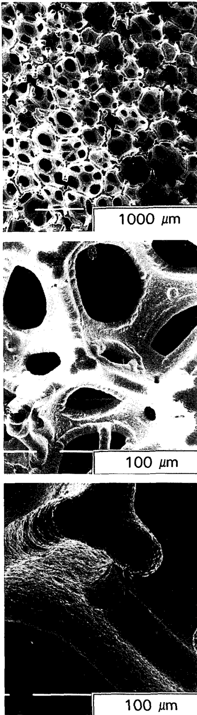
Fig. 6. S.E.M. photographs of nickel plated polyurethane foam.
