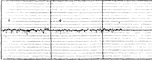
Fig. 6(a). Profilometer trace of M50 rod run for 30 minutes at room temperature, 3200 RPM and a pressure of 5000 Mpa. Lubricated with polyol ester.
