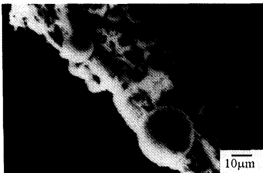
Fig. 10. Small size type II spheres. Some sphere shows eruptive hole on its surface.
