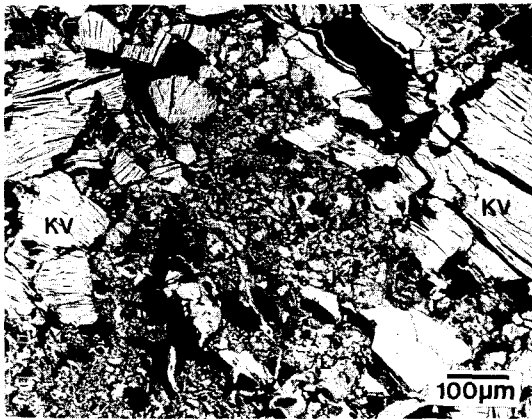
Fig. 8. K-bearing illitic books (K) among the kaolinite-vermiculite pseudomorphs (KV) after biotite.
