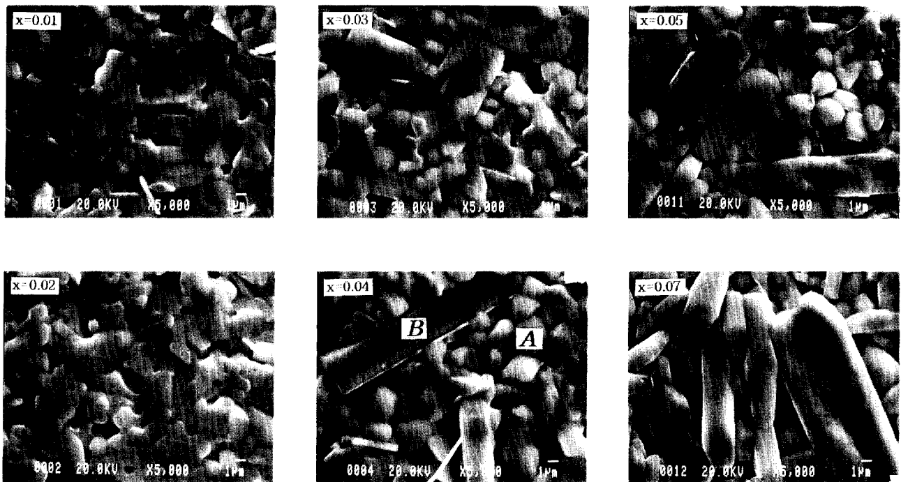
그림 3 1320^\circ\text{C} 에서 4시간 소결한 (1-4x)(\text{BaTiO}_3-3\text{TiO}_2)+4x(\text{Zn}_{1/3}\text{Nb}_{2/3})\text{O}_2 세라믹스의 (\text{Zn}_{1/3}\text{Nb}_{2/3})\text{O}_2 의 첨가량에 따른 미세구조의 변화 Fig. 3 Microstructural changes as a function of (\text{Zn}_{1/3}\text{Nb}_{2/3})\text{O}_2 contents in the (1-4x)(\text{BaTiO}_3-3\text{TiO}_2)+4x(\text{Zn}_{1/3}\text{Nb}_{2/3})\text{O}_2 ceramics sintered at 1320^\circ\text{C} for 4h
