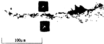
Fig. 3 Indentations near crack tip
