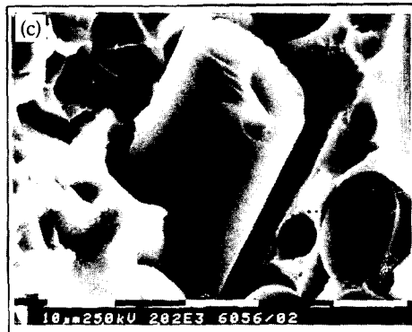
Fig. 6 SEM micrographs of fracture surface of hybrid composites after tensile test (a) overall view and (b), (c) high magnification
