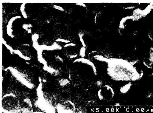
Fig. 7 SEM micrograph of (a) pores ( \times 5,000 ) and (b) microcracks ( \times 5,000 ) in NASICON electrolytes prepared by improper thermal cycling.
