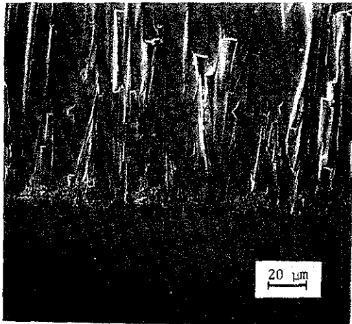
Fig. 2. Cross-Sectional SEM Photomicrograph of the Electron Beam-Physical Vapor Deposited Thermal Barrier Coating Before Cyclic Oxidation Test.
