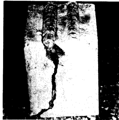
Fig. 5 Split cracking of multiple-bar specimen
