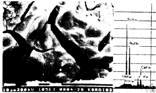
Photo. 7 Scanning electron micrograph and energy-dispersive spectrum of reaction product within mortar bars made with the D aggregate
