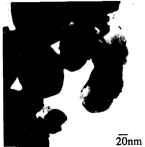
Fig. 9. TEM micrographs of carburized WC/Co powders.
