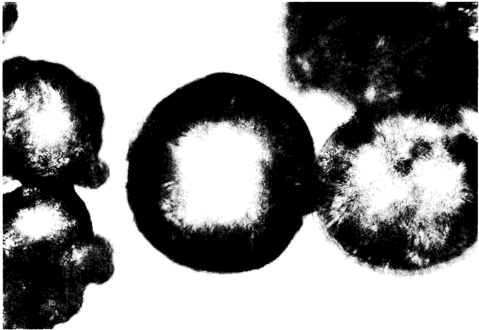
Figure 1. Microphotograph picture of cross-linked chitosan microcapsule using glutaraldehyde (x400)
