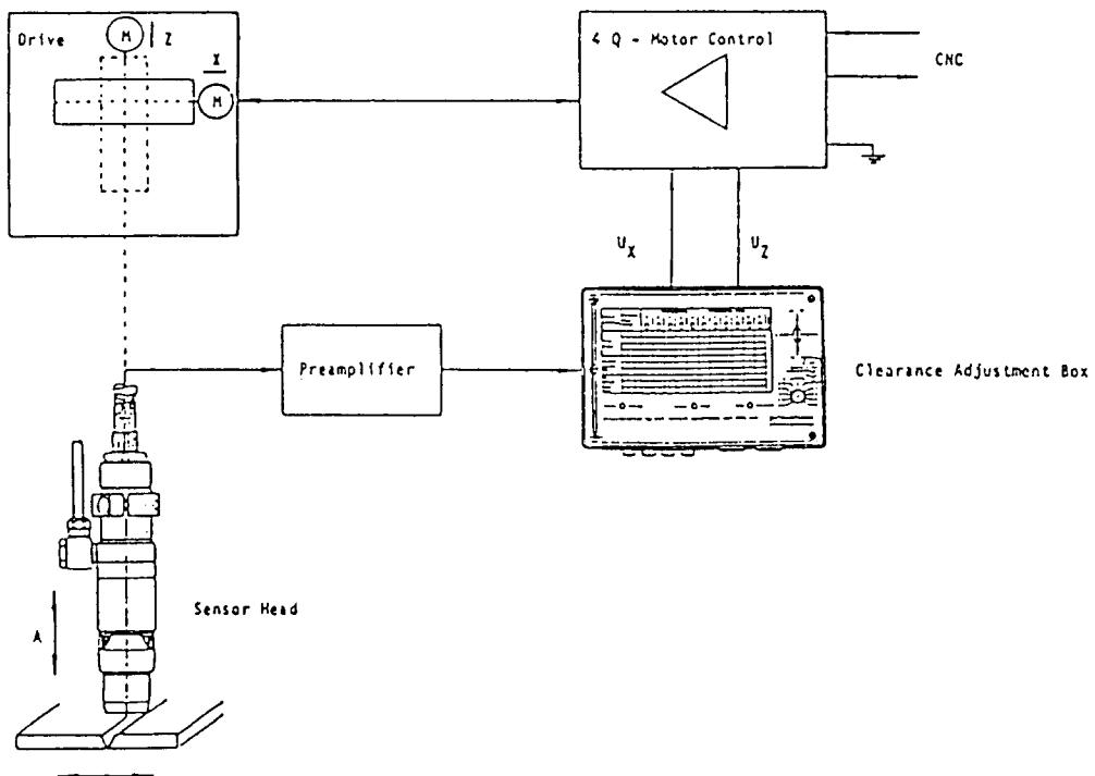
Fig. 2.3 Diagram of a Seam Control System
