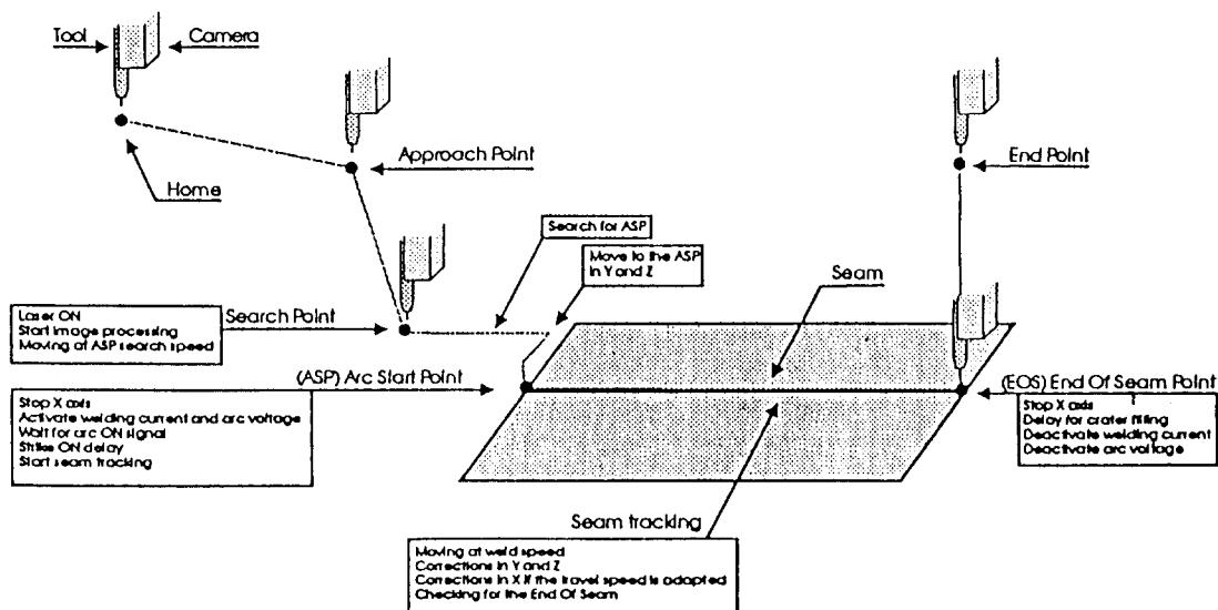
Fig. 2.12 Samkit System Process Cycle
