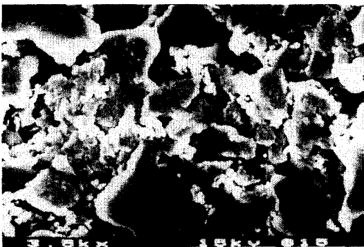
Pho. 1. Scanning electron micrograph of the hydrated portland cement.
