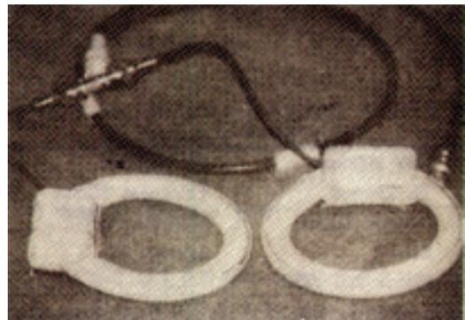
Fig. 3-b Bilateral type 100mm diameter surface coil.
