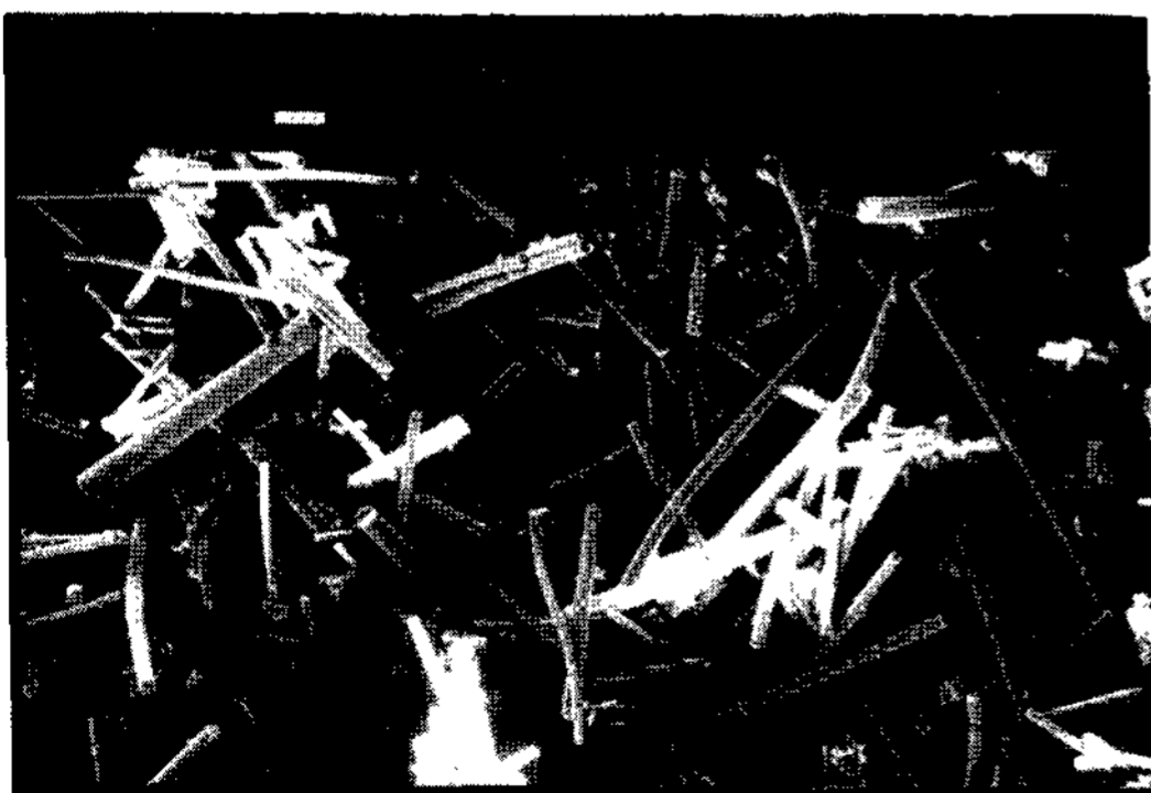
Photo 5. SEM microphotograph of fibers extracted from composite reinforced with 15 vol% Al_2O_3 short fibers after rheo-compocasting, hot pressing and T_6 treatment.
