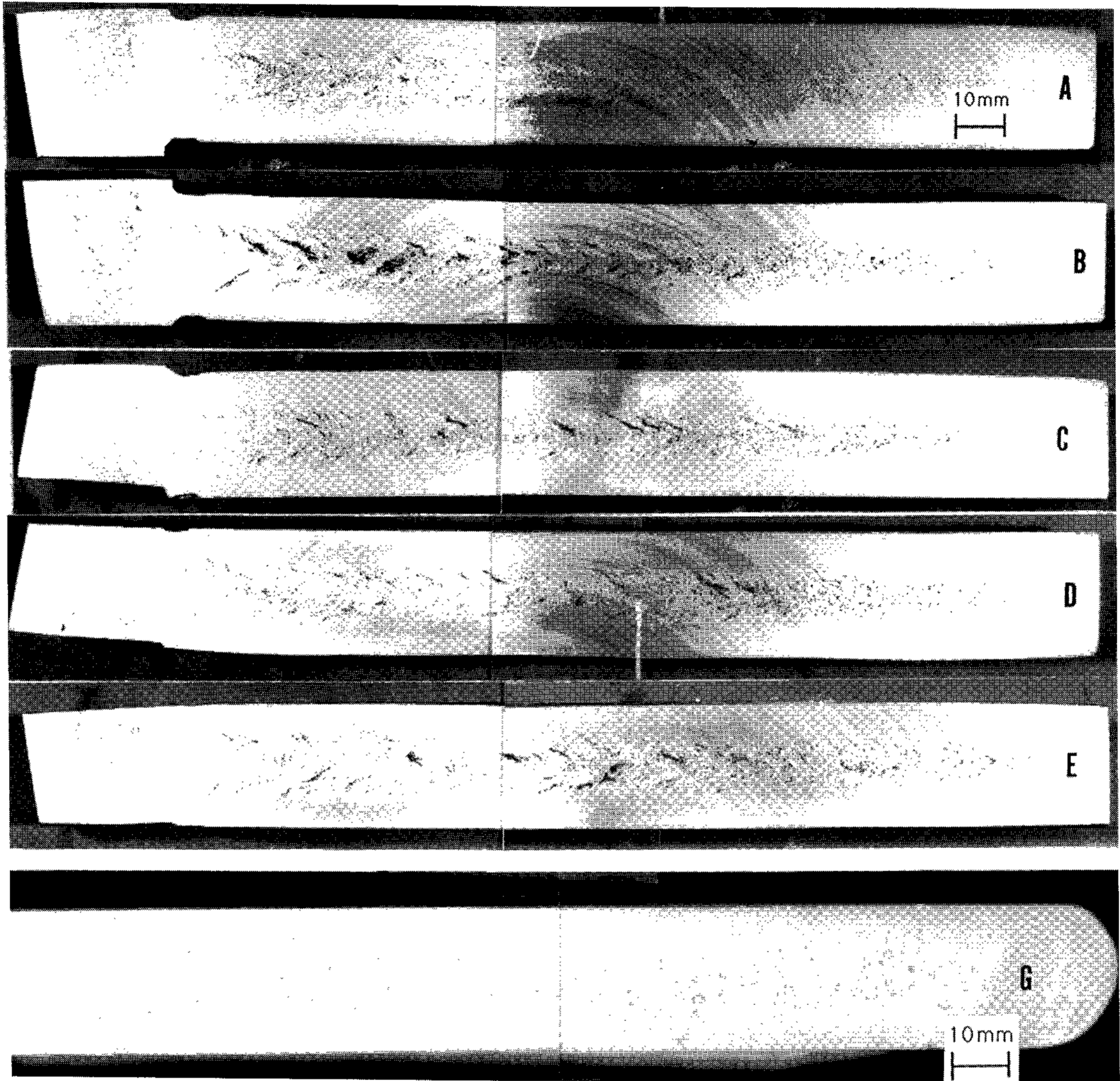
Fig. 7. Macrostructures of longitudinal section under various injection conditions.
