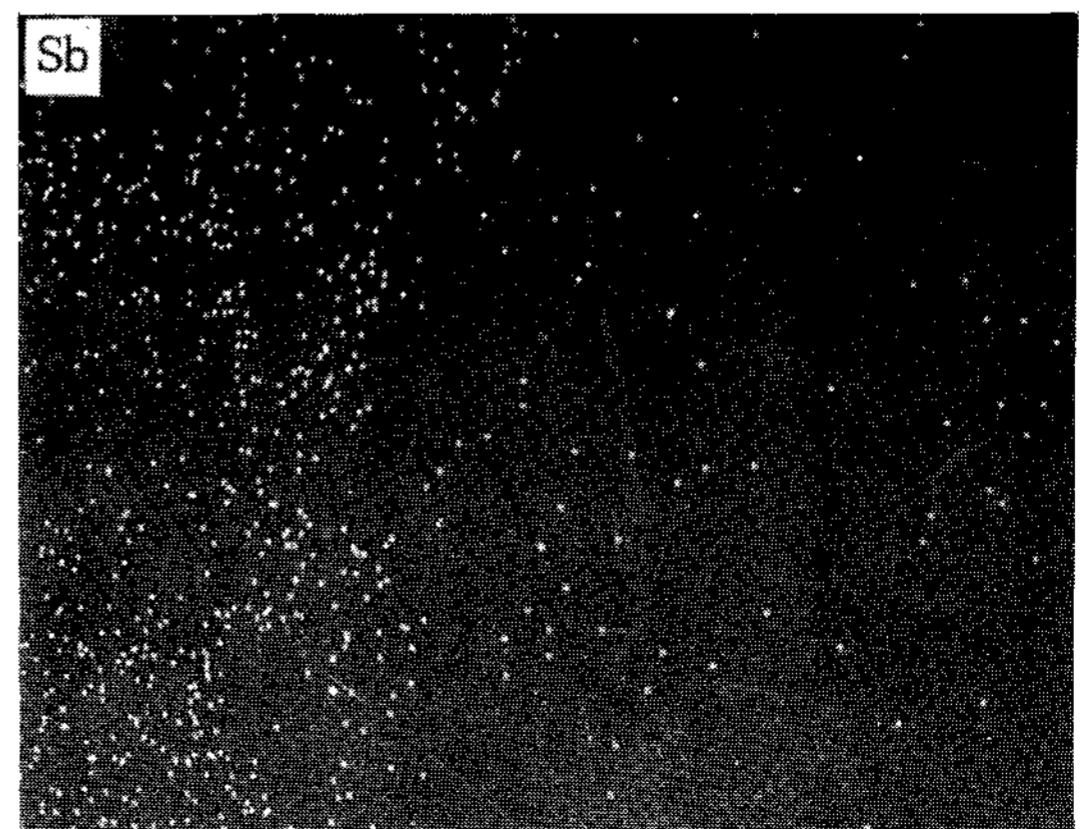
Photo. 5 Microstructure and EPMA(WDX) of bond interface. Mold rotating speed : 1000rpm Pouring temp. of Cu-powder : 1120°C, Babbitt metal : 700°C
