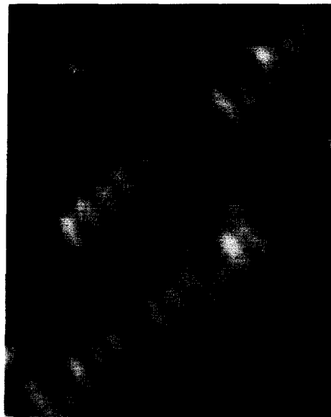
Fig. 3. 150 \times 150 \text{ \AA}^2 image of Ge on Si(100) surface, with Ge coverage of about 0.5 m \ell .
