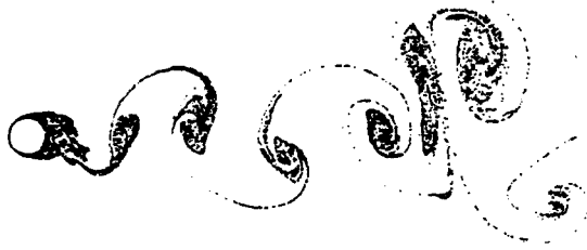
Fig. 6 The vortex distribution pattern at t = 40 with the parameters, \delta = 0.1, \Delta t = 0.2, \xi = 0.03
