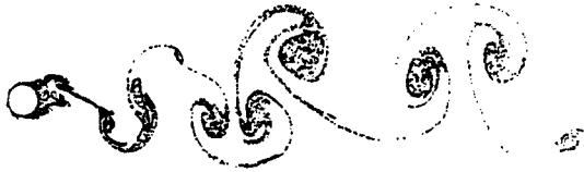
Fig. 4 The vortex distribution pattern at t = 40 with the parameters, \delta = 0.06, \Delta t = 0.2, \xi = 0.04
