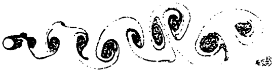
Fig. 7 The vortex distribution pattern at t = 60 with the parameters, \delta = 0.1, \Delta t = 0.2, \xi = 0.05
