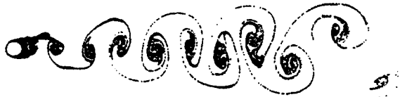
Fig. 3 The vortex distribution pattern at t = 60 with the parameters, \delta = 0.1, \Delta t = 0.2, \xi = 0.04
