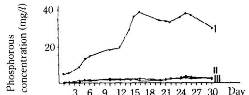
Fig. 6. Release of phosphorous from activated sludge under unaerobic condition.
