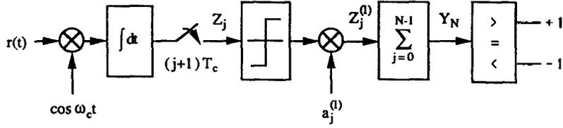
Figure 1. The DS/SSMA hard-limiting correlation receiver
