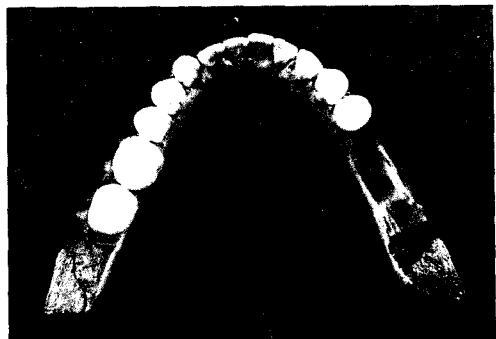
Fig.2. Photoelastic cast coated with plastic cement - 1.
