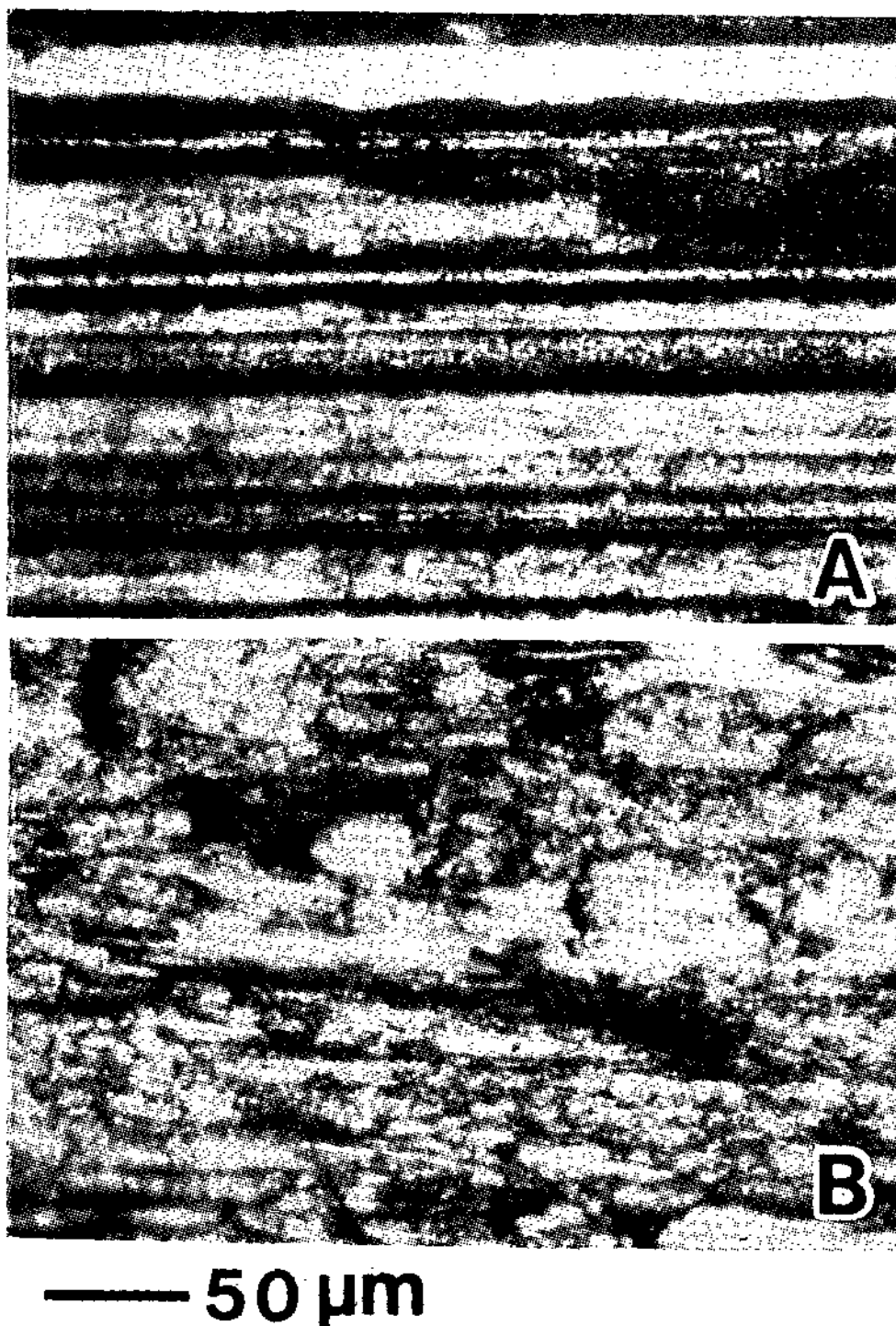
Photo 6. Surface morphologies of Al-4.5 w/o Pb preform worn out with rotation speed of reference material. (A)low speed (B)high speed
