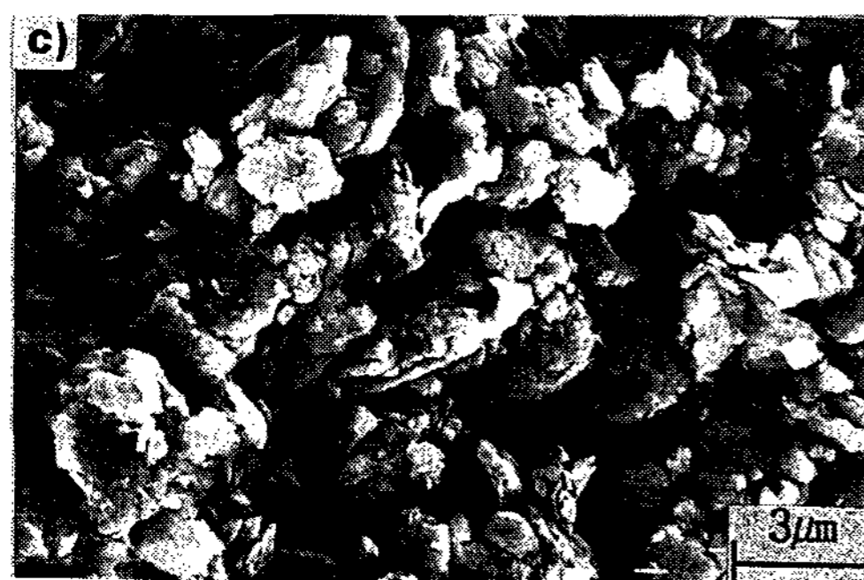
Fig. 12. Scanning electron micrographs and EDS scans of wear debris: (a), (b) PM Cu-graphite (PM1) composite (c), (d) squeeze cast Cu-10%Sn/CF composite.
