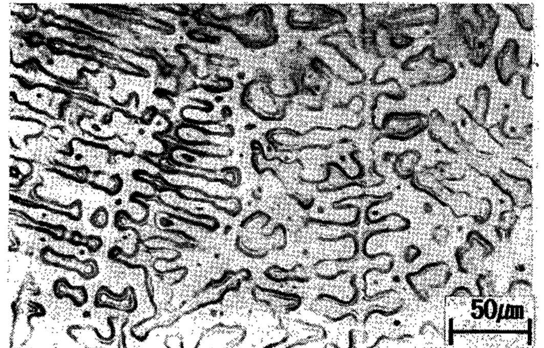
Fig. 3. Microstructure of the unreinforced region(Cu-10%Sn) after squeeze casting in the preheated graphite mold.
