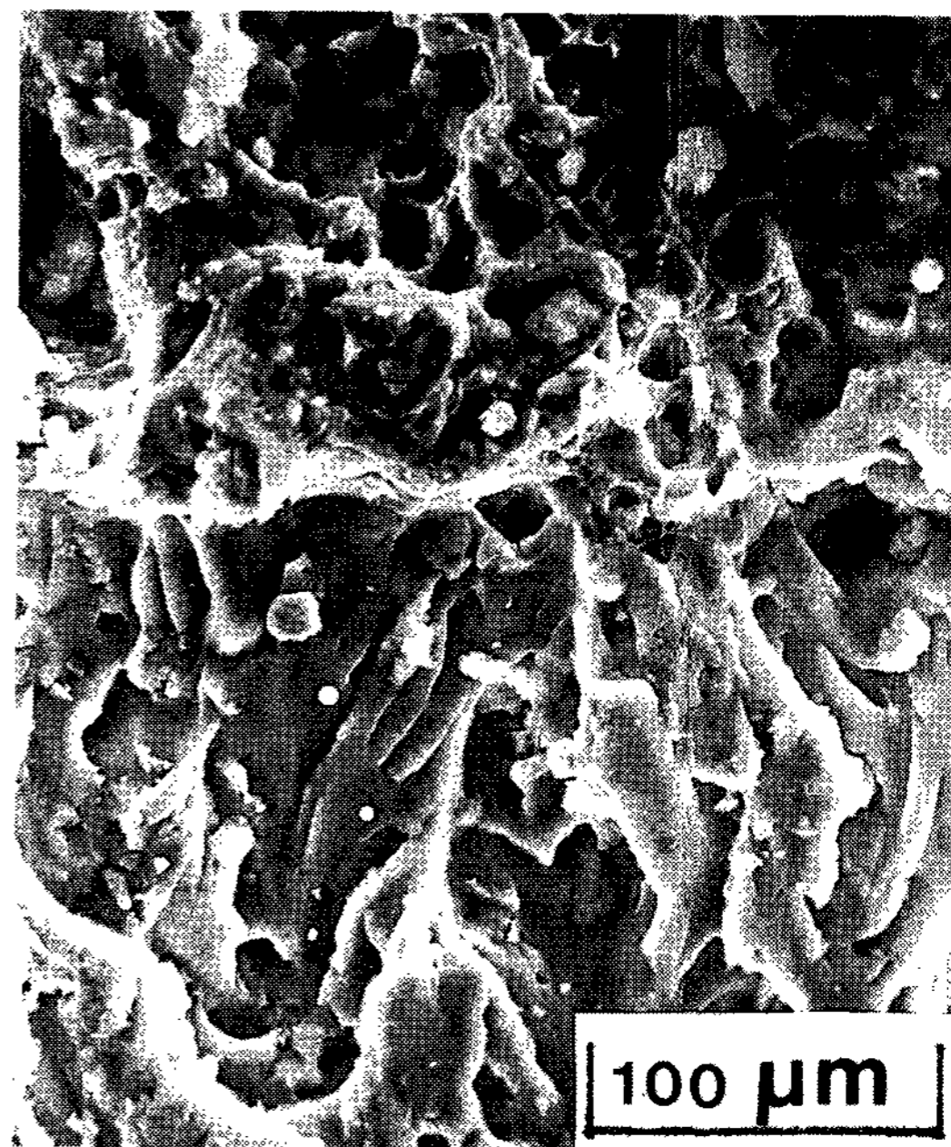
Photo 4. SEM micrographs of fatigue crack surface.
