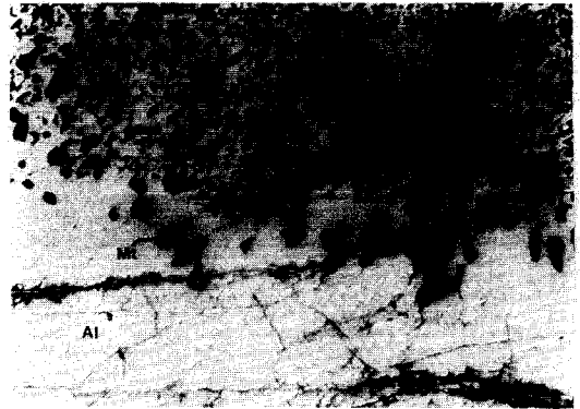
Fig. 4. Magnetite grains(MT) disseminated in the allanite.
