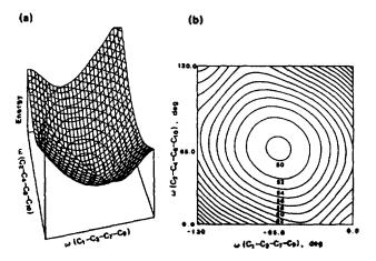
**Figure 1.** MMP2 torsional energy surface of bicyclo[4.2.2]decapentaene with dihedral angles at  $C_1$ - $C_3$ - $C_7$ - $C_9$  and  $C_2$ - $C_4$ - $C_8$ - $C_{10}$  as two variables. (a) Three-dimensional perspective. (b) Contour map. Energies in kcal/mol. See Figure 2 for numbering of atoms.
