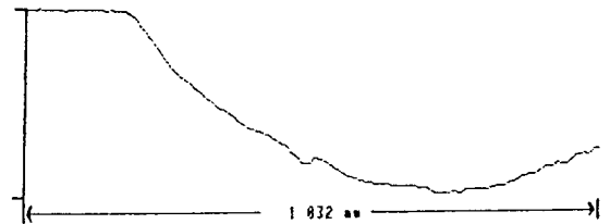
Fig. 24 Profile curve of Taylor-Hobson. Cutting time (20 min)
