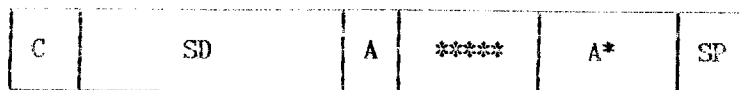
Fig. 1. Freezing apparatus with straw loaded as indicated; C : Cotton plug, SD : Sucrose dilution(7.0 cm), A : Air bubble(0.5 cm), A* : Air bubble(1.5 cm), **** : Vitrification solution+embryos(1.0 cm), SP : Straw powder(0.5 cm)
