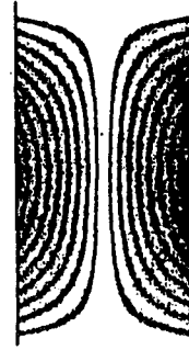
Fig. 4 Example for the vibration mode of a smooth plate
