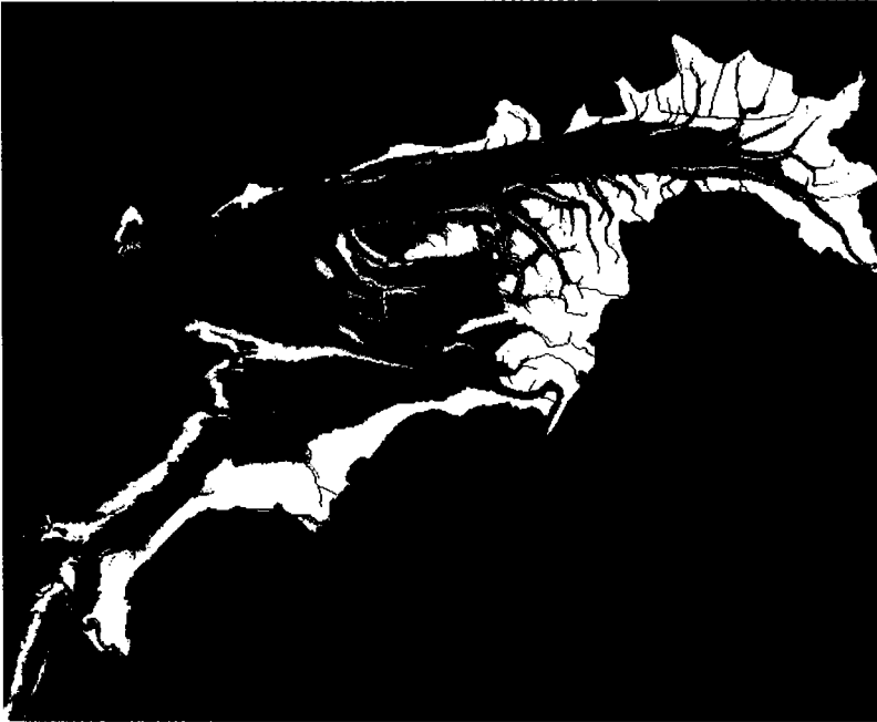
Fig. 6 Extracted color coded contour image by overlapping procedure of nine mask images which show different water height.
