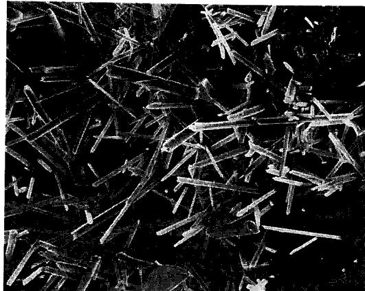
Fig. 11. Scanning electron micrograph of nutrient crystals after hydrothermal growth( $390^{\circ}\text{C}$ ,  $1300\text{Kg/cm}^2$  14d).
