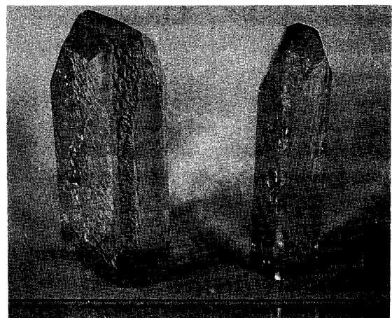
Fig. 7. Photograph of quartz crystal grown in NaOH+LiOH solution.
