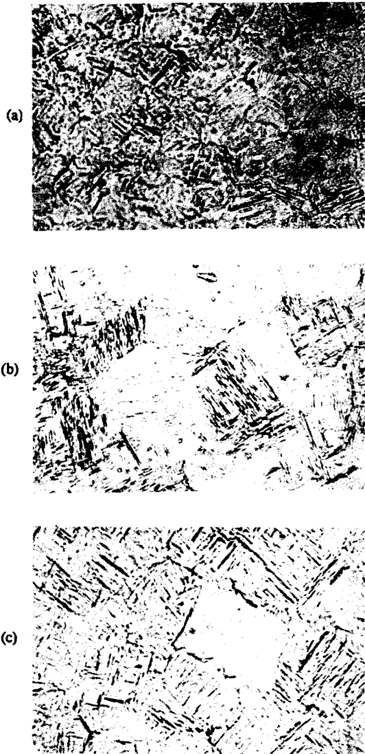
Fig.9 Microstructures of Zircaloy-4 resistance upset welds as a function of main heat (X500). (a) 50%, (b) 60%, and (c)75%
