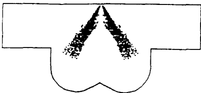
Fig.7 Fuel Droplets Distribution at 130° ABDC for Swirl Ratio 1
