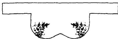
Fig.9 Fuel Droplets Distribution at 150° ABDC for Swirl Ratio 1
