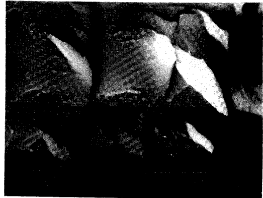
Fig. 7. Matrix Fracture Surface of Carbon/BMI ( \pm 45^\circ ) 2s at Tensile Test. Compimide 800 + DABCO (0.2%).
