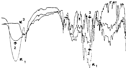
Fig. 4—IR spectra of OMP-complex, physical mixture of OMP and \beta -CD, and OMP.
