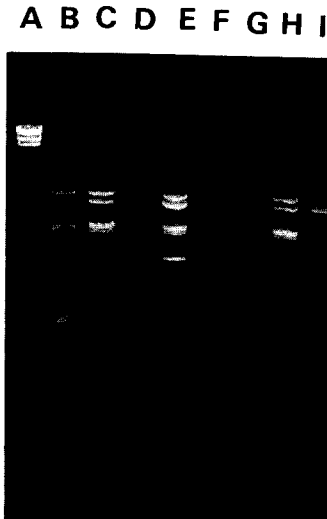
Fig. 3—Electrophoresis pattern of recombinant plasmids from B. subtilis BD170 transformants digested with Sau3AI .
