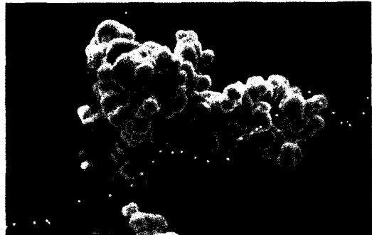
Figure 3—milling. Acetaminophen powder after 6 hrs.
