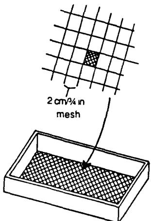
Fig. 3: Testing of Fertilizer After Accelerated Caking Test
