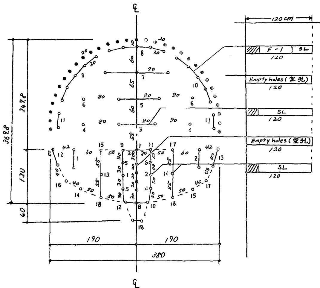
但, Cut holes 은 Tapered Bit  $\phi$  40 mm
