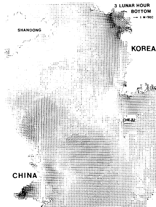
Fig. 14. Computed M_2 tidal current at sea-bottom (3 lunar hour) from the three-dimensional model.
