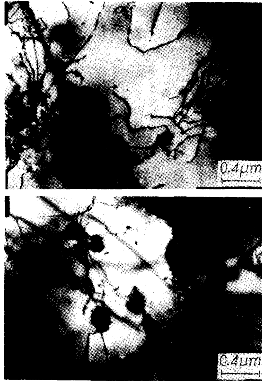
Photo. 1 Distribution of dislocations and precipitates after 1714 hours on 8kgf/mm^2 at 680^\circ C of B1-b specimen
