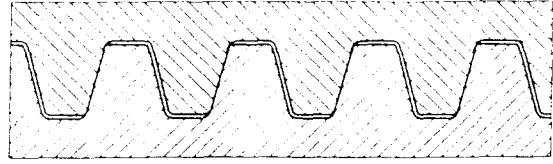
Fig. 3 Acme thread form
